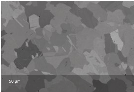
Microstructure from Heat Treatment Option 1. Oxalic acid etch, section perpendicular to building direction.
